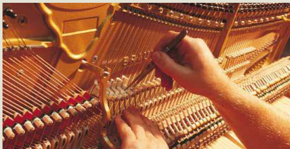
Alignment of the damper drums, to which the felt damper heads, will later be glued (above).
