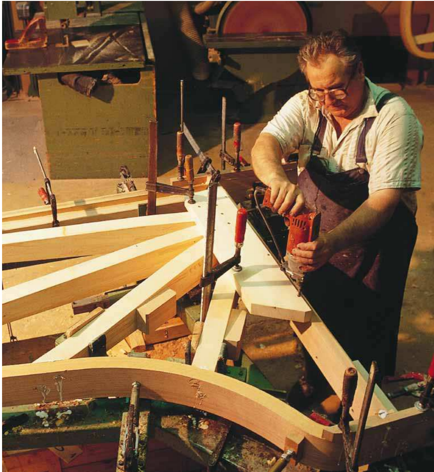
Today strenuous work operations are done by machines, even in piano manufacturing. But most of the work operations are still done by hand and still require a high degree of skill, for example, the assembly of the heavy wooden backframe assembly of a grand.
