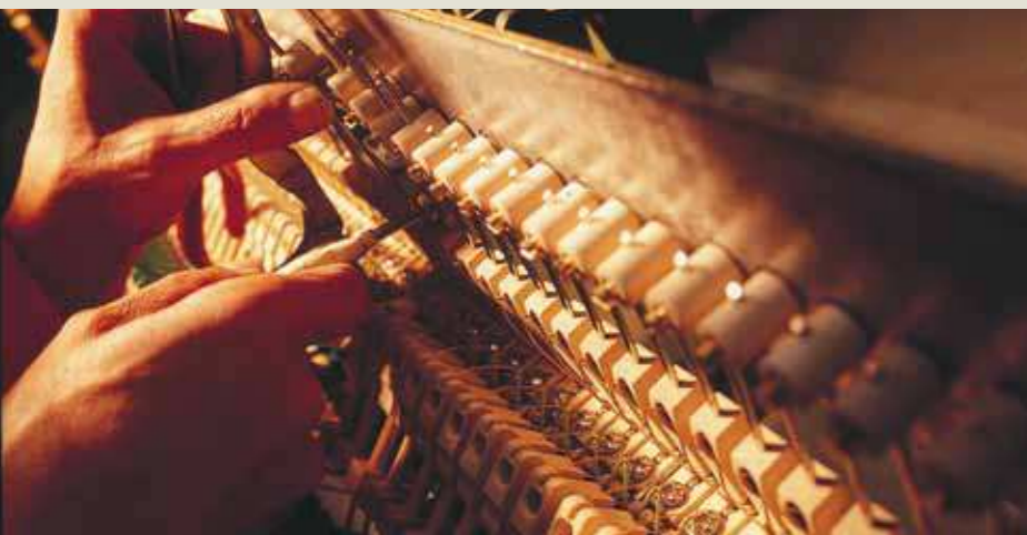
Alignment of the damper drums, to which the felt damper heads, will later be glued (above).
