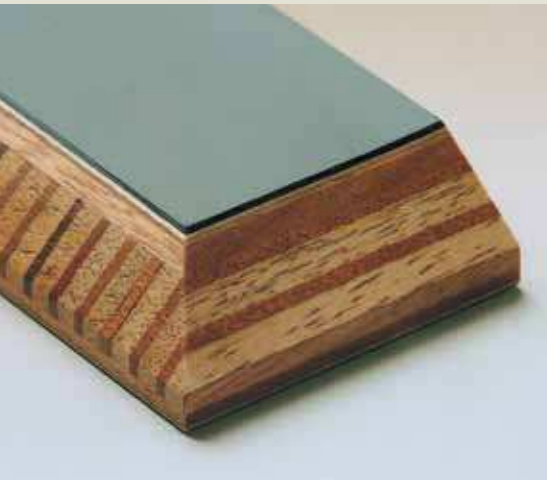
Modern glue technology creates the basis for the manufacturing of laminated-wood stock, which in piano manufacturing is used for components requiring a high degree of durability.
