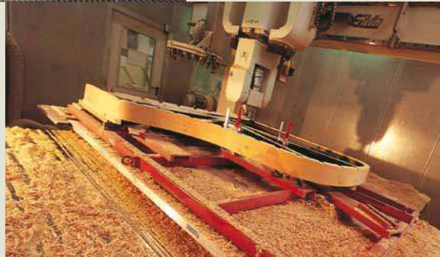
Exact to a hundredth of a millimeter, the Schimmel CNC-controlled machining centers assure precision in wood and steel machining.
