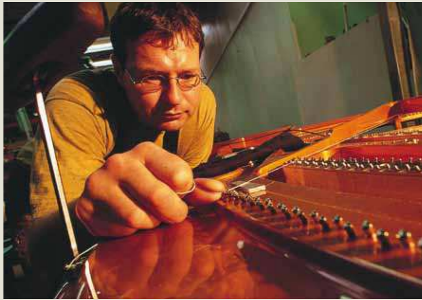
Tone quality is the result of know-how and precision at all stages of the production process. Which is why at Schimmel care is cultivated everywhere – as in the checking of the height of a bridge in relation to the plate (above) and the first-chipping operation (below).
